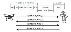
Figure 2. D2GCS communication and packet structure.
