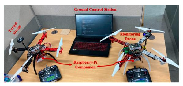
Figure 9. The actual experimental testbed for the proposed security protocol.
