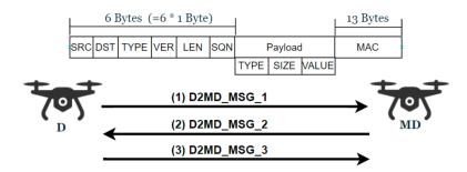
Figure 4. D2MD communication and packet structure.
