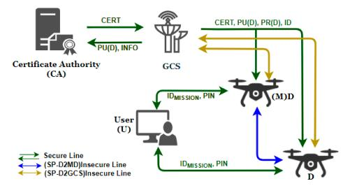
instance PIN), IP address, type of UAV (monitoring or general drone), and operation ID (ID<sub>MISSION</sub>) are configured by the user before the UAVs start their mission.
